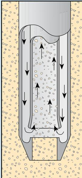
The Rakoraf "Core Sampler" is the fastest and easiest method to take an accurate sample from an open trailer. The sample is taken while the trailer is still on the weighbridge.
