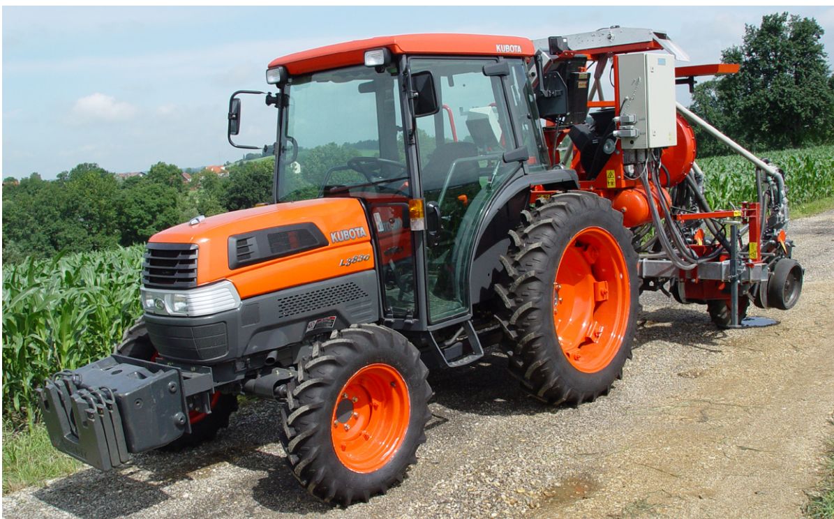
Plot tractor Kubota L5030 with cabin and plot precision planter Hege 95:
