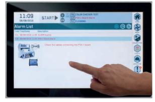
Alarm smart explanation for immediate repair
