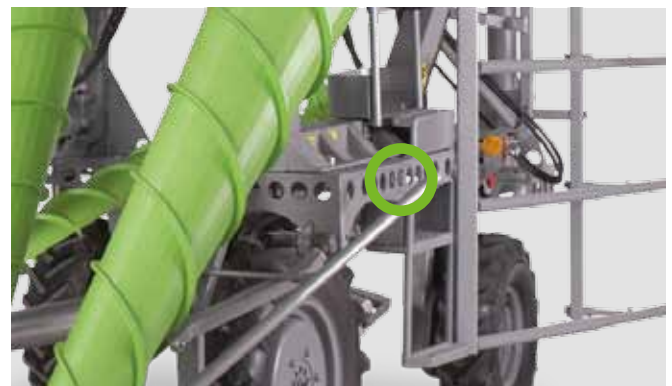
Screws on the front axle for adjusting track width
