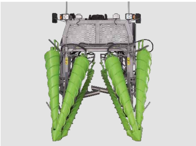
4 torpedoes mounted above and 2 below along with 2 horizontal pressure rolls
