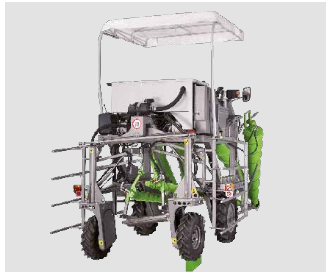
Rear wheel suspension with full floating axle for a high degree of adaptability
