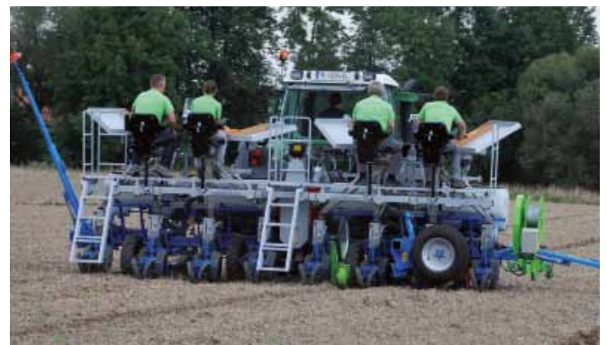
WINTERSTEIGER Dynamic Disc on 8-row tractor mounted frame (3-point or pull type design available)
