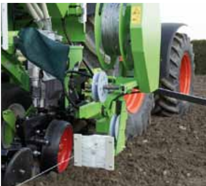
Cable trip system with cable winder
