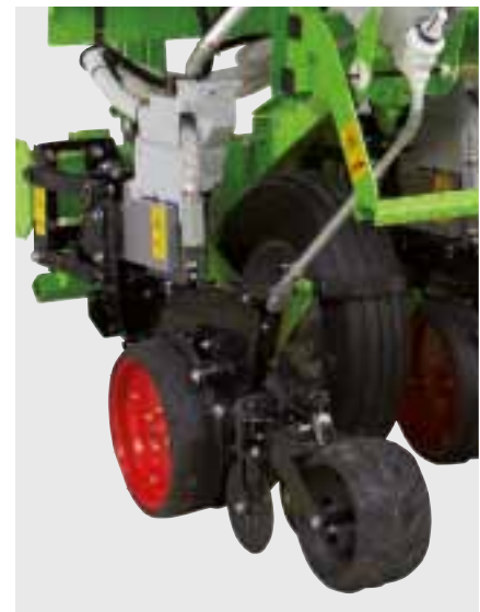
Compact processing of the electric drive on the seed unit
