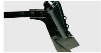
NODET shoe opener, row spacing as of 8.5 cm, deposition depth max. 4 cm, depth guide via sowing depth restrictors
