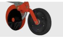
ACCORD CX single disk opener, row spacing as of 9.5 cm, deposition depth max. 5 cm, depth guide via pressure roller
