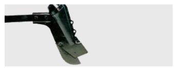
NODET shoe opener, row spacing as of 8.5 cm, deposition depth max. 4 cm, depth guide via sowing depth restrictors
