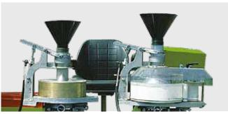
Øyjord cell wheel system and belted cone placed side by side for simultaneous sowing and fertilizing
