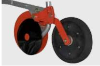
ACCORD CX single disk opener, row spacing as of 9.5 cm, deposition depth max. 5 cm, depth guide via pressure roller
