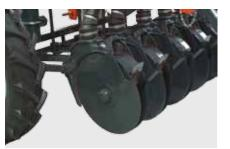
NODET double disk opener, row spacing as of 10 cm, deposition depth max. 8 cm, depth guide via pressure roller
