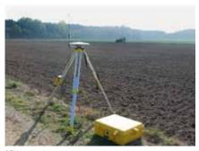
RTK station for maximum precision sowing
