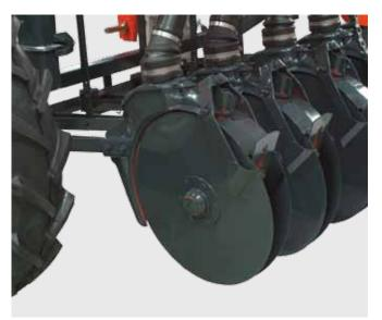
NODET double disk opener, row spacing as of 10 cm, deposition depth max. 8 cm, depth guide via pressure roller
