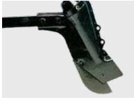
NODET shoe opener, row spacing as of 8.5 cm, deposition depth max. 4 cm, depth guide via sowing depth restrictors
