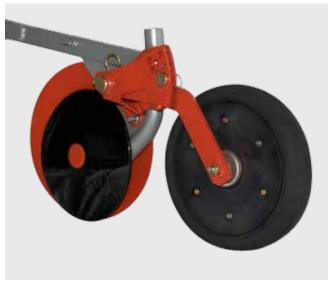
ACCORD CX single disk opener, row spacing as of 9.5 cm, deposition depth max. 5 cm, depth guide via pressure roller
