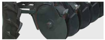
NODET double disk opener, row spacing as of 10 cm, deposition depth max. 8 cm, depth guide via pressure roller
