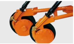
AMAZONE RoTec roller opener, row spacing as of 12.5 cm, deposition depth max. 4 cm, depth guide via stop
