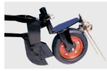
WINTERSTEIGER shoe opener, row spacing as of 10 cm, deposition depth max. 4 cm, depth guide via FARMFLEX pressure wheel
