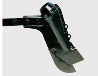
ISARIA shoe opener, row spacing as of 8 cm, deposition depth max. 4 cm, depth guide via pressure roller
