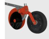
ACCORD CX single disk opener, row spacing as of 9.5 cm, deposition depth max. 5 cm, depth guide via pressure roller
