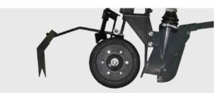
ISARIA shoe opener, row spacing as of 8 cm, deposition depth max. 4 cm, depth guide via pressure roller
