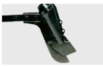
NODET shoe opener, row spacing as of 8.5 cm, deposition depth max. 4 cm, depth guide via sowing depth restrictors
