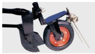
WINTERSTEIGER shoe opener, row spacing as of 10 cm, deposition depth max. 4 cm, depth guide via FARMFLEX pressure wheel
